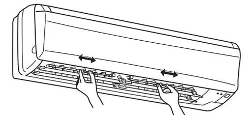
Adjust the vane before operation starts. Since the horizontal vane moves automatically, your fingers may be caught.
